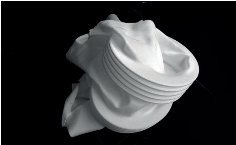
Multiple parallel lines self-organizing into a tube/roll.
