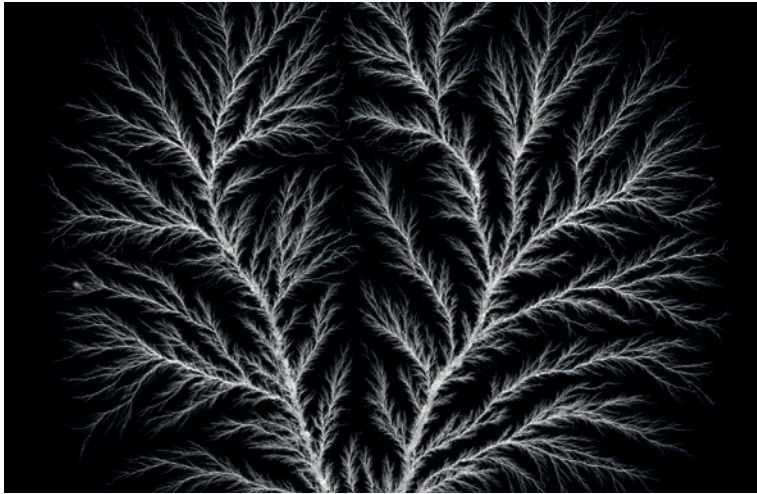
Emile De Visscher, electrical treeing by partial discharge of a PMMA block, detail. Conducted at LSI Lab, École Polytechnique. Thanks to EMIR&A research network. 2021, @Palta Studio.
