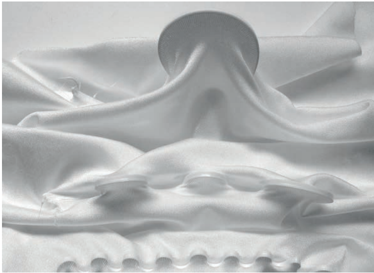
How to control the wavy shape of 3D printed lines. Left: Influence of line thickness (increasing from bottom to top); Right: Influence of textile pre-stretch (increasing from top to bottom).
