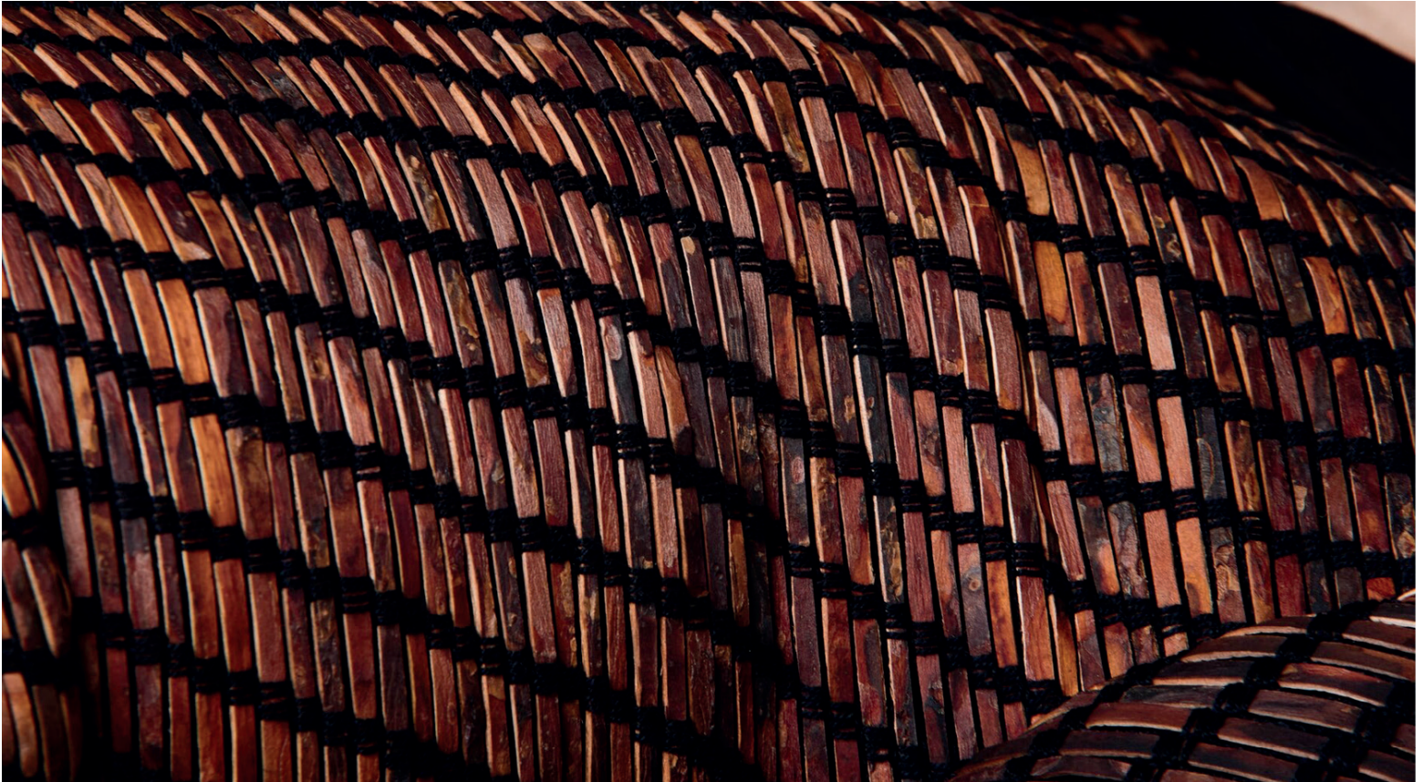
Twill weave was used for textile applications made out of bark. First tests showed a better superior and were used for a woven bark jacket.
