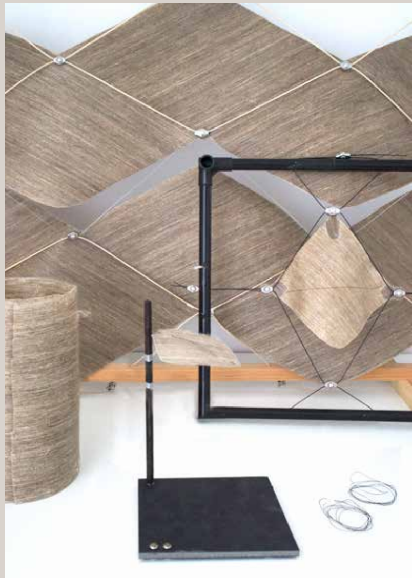
Modular shading with shape memory alloy and biobased textile membrane. Photo: Maxie Schneider
