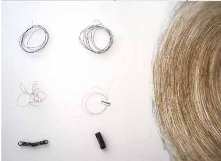
Designing polymorph textility by fusing fiber based materials shape memory alloy actuators and biobased membranes (bottom) to achieve bistable elastic modules (middle) for adaptive urban shades (top). Photos: Maxie Schneider
